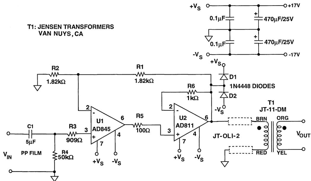
**Figure 6-58:** A basic transformer coupled line driver
