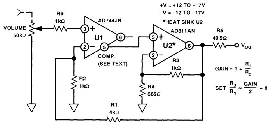
**Figure 6-51:** Composite current boosted line driver one
