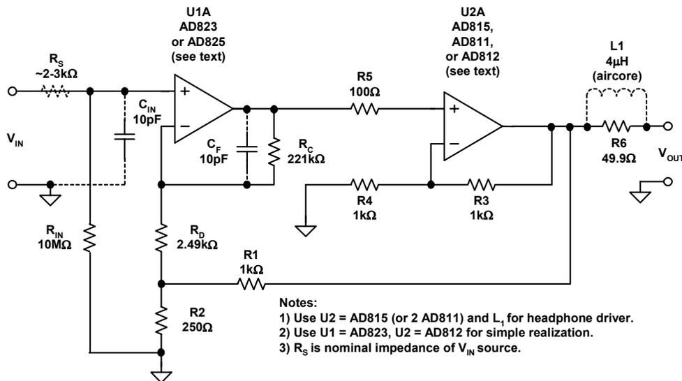
**Figure 6-53: Composite current boosted line driver two**
