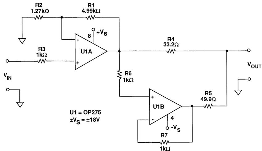
**Figure 6-45:** Paralleled output dual op amp line driver
