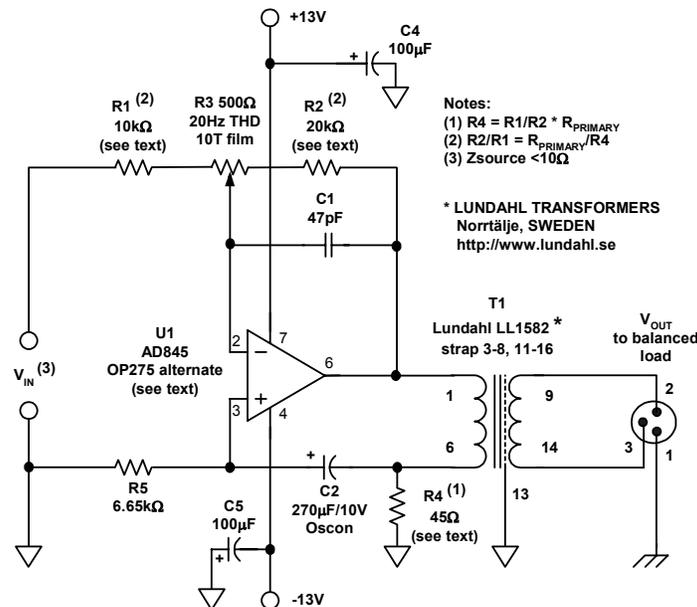
**Figure 6-61:** A basic single-ended mixed feedback transformer driver
