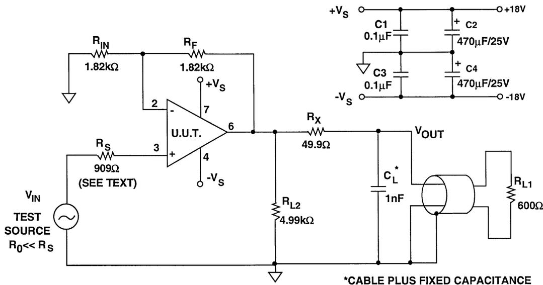
**Figure 6-39:** Test circuit for audio line driver amplifiers
